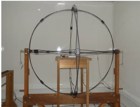
7.3. Photo of radiated emission measurement (R.E. Electric field)
